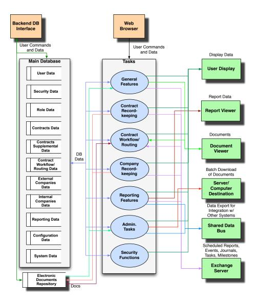
The above diagram shows the main "Tasks" or functionality areas of the system from the Data Flow Diagram Level 1 in the Requirements document. The diagram also shows the Main database on the right, and then data output areas on the left. Note that the diagram has been somewhat modified for simplicity in that External/Internal Company Management functionality will be considered part of the Company Record-keeping area.
